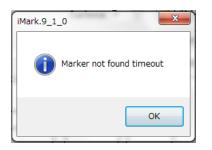
When this message is displayed, click "OK" button on the message window, the media that fed to the CE7000-40 automatically ejects to the F-Mark2.
