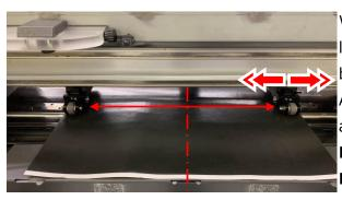
When loading the calibration sheet into the CE7000-40, load the calibration sheet so that the it is centered between the left and right Push Rollers. And change the position of right side Push Roller according to the width of calibration sheet. **NOTICE**
