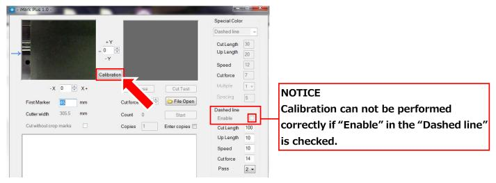
4. The "Calibration" window will be displayed, then click the "Cut Marker" button, and then the CE7000-40 will be cutting a small square on the Calibration Sheet.
