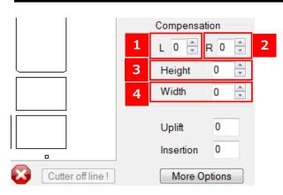
The printed images with digital printer are often distorted. The iMark Plus software uses the optical camera to detect the crop marks to corrects distortions in the printed images near the crop marks and to corrects the cutting position.
